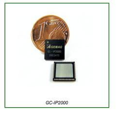
The interpolation circuit GC-IP2000 serves to increase the resolution for incremental position and angular measuring systems with sinusoidal output signals offset by 90°. The IC divides the signal period up to 2,048 times.
