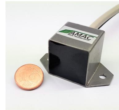
The AM-SW1D is a vibration and shock sensor system with an integrated mixed signal circuit AM-CVC2D. The system delivers via the serial interface the digital measurement of the calibrated sensors for vibration (8k) and shock (20k). FIR parameters, temperature, and monitoring data such as threshold parameters can be also send via the SPI/CAN serial interface. The resolution/sensitivity of the sensor is also programmed and set according to specific requirements\*.
